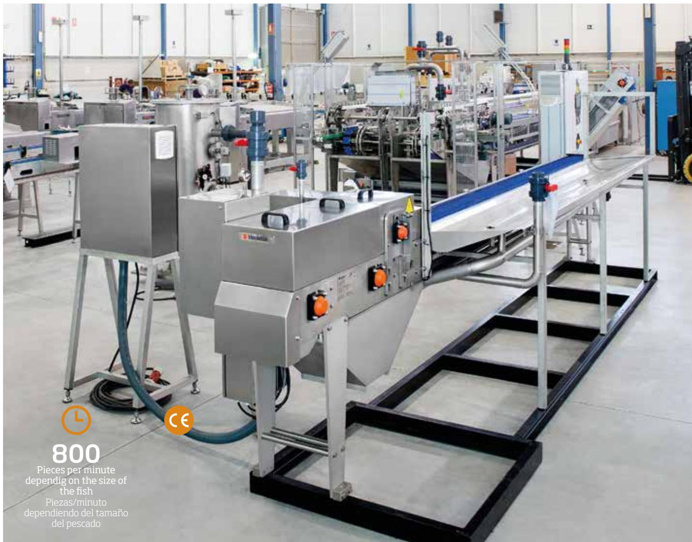
Machines designed for continuous de-heading and removing tails and gutting sardines or similar species.
